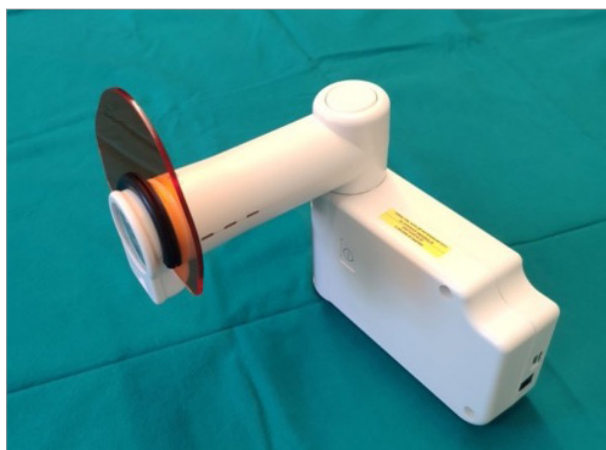
Figure 1. The medical device (EmoLED) used for Photobiomodulation with blue LED light
